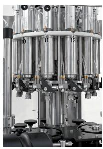
Of the entire bottling line, the most important unit is the filling machine. The filling unit is the only component that has direct contact with the finished product and therefore must be conceived, designed and built so it provides utmost reliability in terms of product guarantee. It must maintain product characteristics during the actual filling operation while being easily washable and sterilizable when in contact with products particularly sensitive to contamination.
