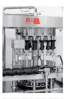
The gravity filling machine can operate by simple gravity and, if the type of container permits, also with a slight vacuum in the tank which, in some cases, helps trigger the actual filling phase.
