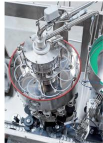
FIMER high-vacuum filling machines are designed specifically for particularly dense products filledinto glass containers or non-collapsible materials, such as miniature PET bottles. The high-vacuumfilling machine operates thanks to a pressure difference.
