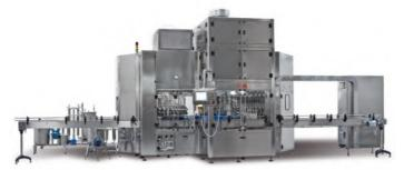
The etymology of the word monoblock immediately conveys a clear idea of what it means; a set of machines forming part of the same block. In the case of the machines made by FIMER, the term "monoblock" identifies a machine integrating the functions of rinsing, bottle filling, corking and capping of various closures.
