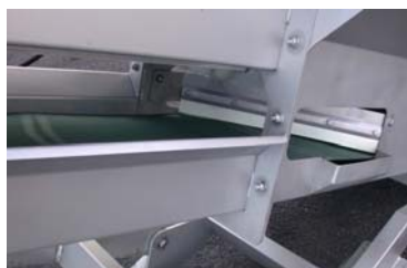
Cleaning rubber below belt
