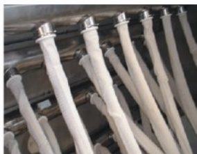
DRAINAGE ELEMENTS INSIDE PRESS
